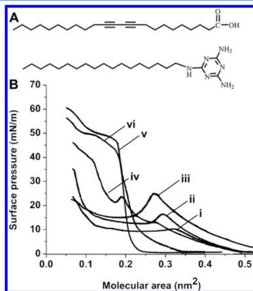
**Figure 1.** Thermodynamic profiles of mixed diacetylene/octadecyl melamine Langmuir monolayers. (A) Molecular structures of diacetylene monomer TrCDA (top) and OM (bottom). (B) Surface pressure/area isotherms of mixed TrCDA/OM Langmuir monolayers at different mole ratios between the two components: TrCDA/OM mole ratios of 6:1 (ii), 3:1 (iii), 1:1 (iv), and 1:3 (v) as well as pure TrCDA (i) and OM (vi).
