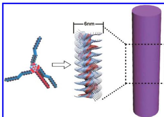
**Figure 5.** Structural model for the assembly of diacetylene/octadecyl melamine nanowires. Space-filling model on the left showing the hydrogen-bonded diacetylene/OM unit. The diacetylene/OM building blocks are stacked through  $\pi$ - $\pi$  interactions, forming the backbone of the nanowire on the right.
