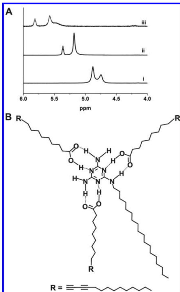
**Figure 2.** Hydrogen bonding between melamine and diacetylene monomers. (A) Amine proton region of the NMR spectra recorded for TrCDA/OM mixtures prior to deposition at the air/water interface: pure OM (i); 1:1 mol ratio between TrCDA and OM (ii); and 3:1 mol ratio between TrCDA and OM (iii). (B) Model for the hydrogen-bonding network assembled between melamine and three TrCDA residues.
