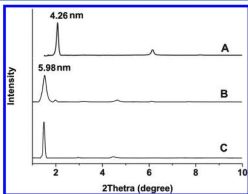
**Figure 6.** X-ray diffraction (XRD) patterns of diacetylene/octadecyl melamine films. (A) Pure TrCDA film. (B) TrCDA/OM (3:1 mol ratio). (C) TrCDA/OM (1:1 mol ratio).
