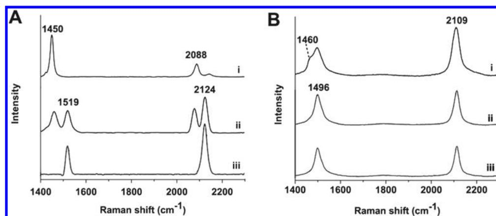
**Figure 8.** Raman scattering peaks in the conjugated alkyne–alkene spectral region of (A) a pure PDA film and (B) a diacetylene/OM film (1:1 mol ratio). (i) UV irradiation for 30 s. (ii) UV irradiation for 40 min. (iii) Heating to 70 °C for 30 min.
