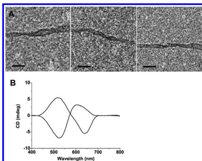
**Figure 4.** Helical organization of the TrCDA/OM nanowires. (A) Transmission electron microscopy (TEM) images showing TrCDA/OM nanowires; the helical pitches are apparent. Scale bars correspond to 50 nm. (B) Circular dichroism (CD) spectra of TrCDA films transferred from the air/water interface. The film chirality gave rise to CD signals (two polarizations recorded for two film samples).
