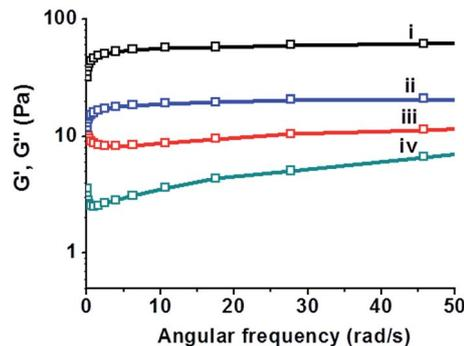
Fig. 4 Bacterially-induced changes to the rheological properties of the C-dot-hydrogel. Angular frequency sweep experiments of C-dot-hydrogel before and after addition of *B. cereus* ( $10^8$  cells per mL) at 37 °C: (i) the storage modulus  $G'$  before addition of bacterium suspension; (ii)  $G'$  after addition of bacterium suspension; (iii) the loss modulus  $G''$  before addition of bacterium suspension; (iv)  $G''$  after addition of bacterium suspension.
