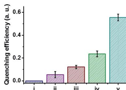
Fig. 7 Quenching of C-dot-hydrogel fluorescence by different bacterial stains. Degrees of fluorescence quenching ( $\lambda_{\text{ex}}$ :  $375\text{ nm}$  and  $\lambda_{\text{em}}$ :  $430\text{ nm}$ ) of the C-dot-hydrogel upon addition of different bacterial species ( $10^8$  cells per mL). (i) C-dots-hydrogel (control); (ii) *Pseudomonas aeruginosa* PAO1 wild type; (iii) *Bacillus subtilis* (stain *Bacillus* 3610); (iv) *Staphylococcus aureus* wild type; (v) *Bacillus cereus*.
