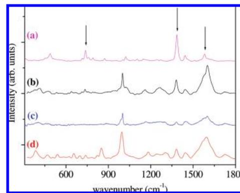
**Figure 2.** Representative SERS spectra of the (a) free template (*S*)-propranolol, (b) molecularly imprinted polymer (MIP), (c) extracted MIP, and (d) after rebinding of the template to the MIP. All the spectra are of samples deposited on the Klarite surface and were measured with integration times of 40 s. The background has been subtracted, and the spectra are plotted on the same scale and are shifted for clarity.
