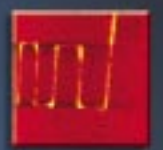
30x30 \mu\text{m} AFM image of a BSA protein line printed using a Nanonics Nanopipette NanoFountainPen™.
