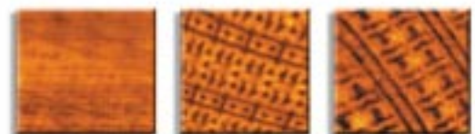
12x12µm images of a SRAM after CMP. The left side shows an AFM image, where almost no structure can be seen. In the reflection NSOM image in the middle, clear structures are visible, caused by differences in the index-of-refraction. The image on the right shows an electrical resistance image.
