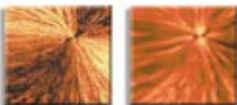
15x15µm images of PEO spherulite. The AFM image (on the right) shows the nucleus and the lamellar crystallites. The transmission, polarization NSOM image shows the radial dependence of the birefringence (butterfly pattern).
