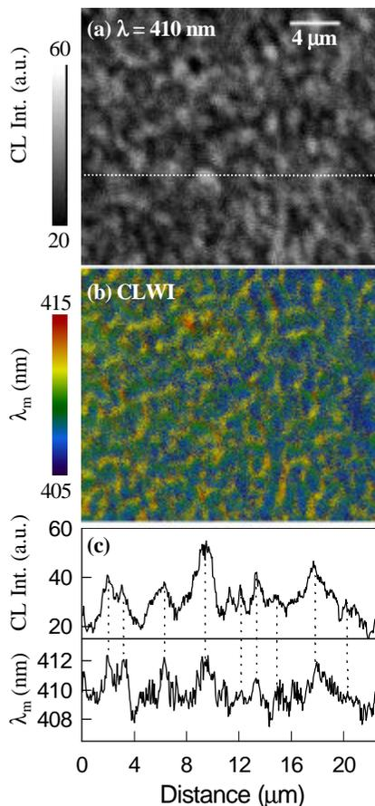
Figure 2. Monochromatic CL image (a), CLWI image (b), and line scan analysis (c) for an e-beam current of 1 nA.
