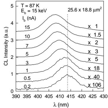
Figure 1. Stack plots of normalized CL spectra for the InGaN/GaN QW sample using various probe currents.
