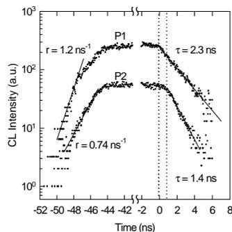
Figure 3. CL transients including the onset and decay near P1 and P2 regions.
