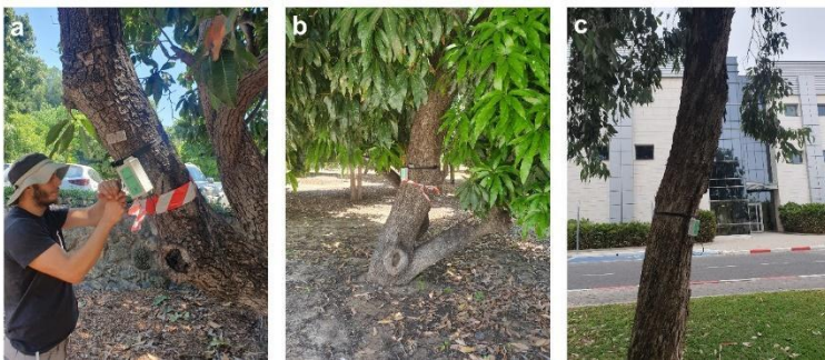
Figure P6. Tree carbon uptake monitoring examples. (a) sensor installation on a tree stem; (b) application on a mango tree in an orchard context; (c) application on a eucalypt tree in a city park context.
