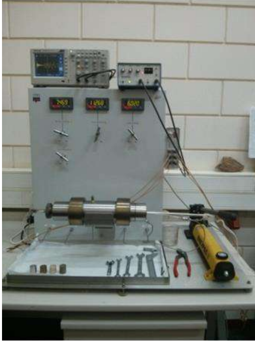
Figure 7: The AVS350 system for P- and S-wave velocities measurements. The stress waves are induced by piezoelectric transducers, oriented in such way to induce compression and shear distortions in the plug. The waves pass through the tested plug and two stain-less steel end caps (one on each side). The stress waves are translated back to an electric current, and arrival times of the waves are picked in the oscilloscope. To identify shear waves in the oscilloscope, the S-wave transducers S1 and S2 are rotated for polarization (transition from (a) to (b) in the sketch).
