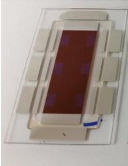
Natural sunlight aging (Nov 15<sup>th</sup> 2015- Feb 21<sup>th</sup> 2016) shows no degradation after >100 days, until the encapsulation broke.
