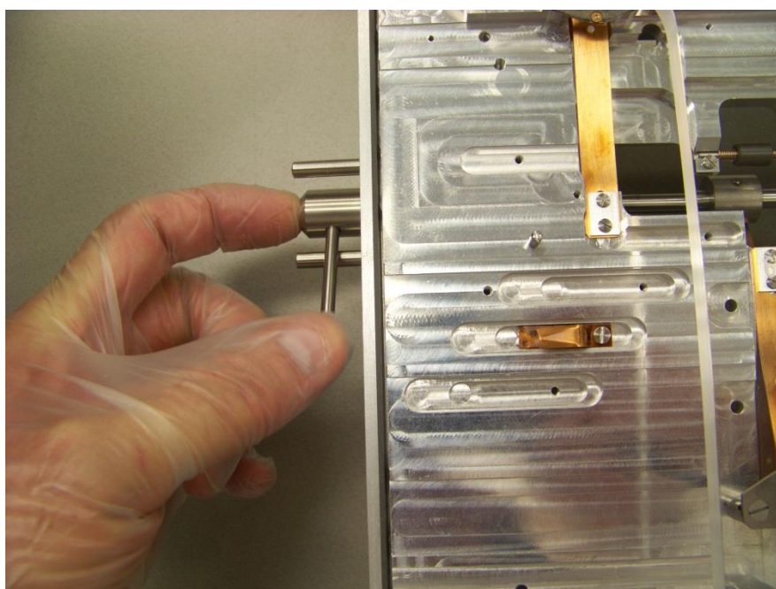
Figure 4 - locking the holder to the loading jig with lever (EBPG5200).
