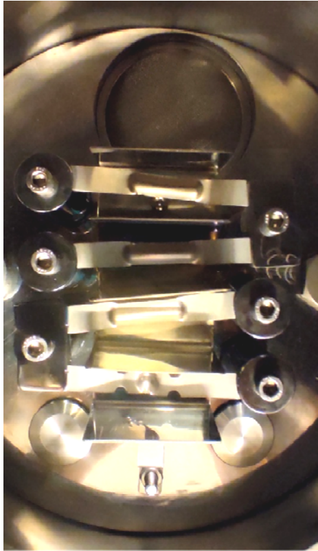
Base Plate with four High-Temp thermal sources
