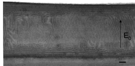
FIG. 11. TEM cross section of thin-film PS-PMMA block copolymer annealed in electric field E_0 \approx 40 \text{ V}/\mu\text{m} . Few lamellae lie parallel to the substrate (bottom) and polymer-air interface (top), while the rest of the film has lamellae parallel to the field. Adapted from Xu, Zhu, et al., 2004.
