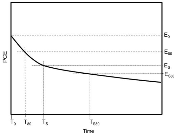
**Fig. 7.** Representative figure defining the parameters to be included in the reporting of OPV stability data. The time evolution of a given parameter of an OPV device, illustrating the four (4) pairs of necessary parameters to describe the decay pattern, including  $E_0$  and  $T_0$ ,  $E_S$  and  $T_S$ ,  $E_{80}$  and  $T_{80}$ , and  $E_{S80}$  and  $T_{S80}$ . Each parameter is defined in text.
