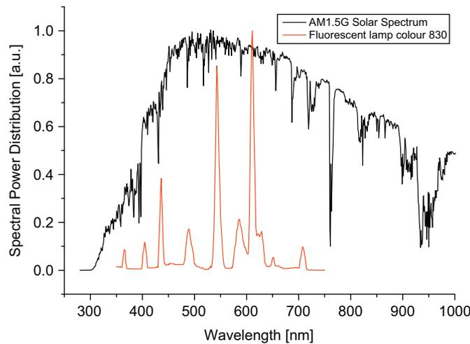
Fig. 4. Comparison of the spectrum of a fluorescent lamp with the light color 830 and the AM1.5 spectrum of the sun.
