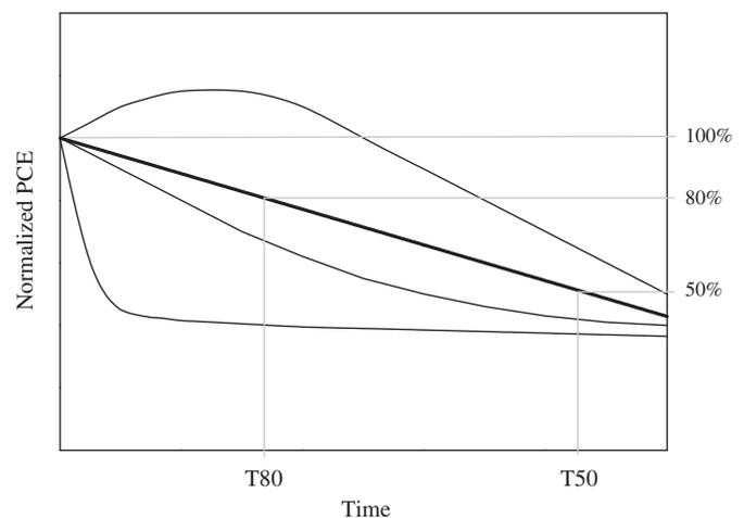
**Fig. 1.** Examples of how the power conversion efficiency for an organic solar cell can evolve with time during operation. The  $T_{80}$  and  $T_{50}$  are shown for a device showing linear decay. Three other examples of commonly observed decay curves are also presented (an increase in performance followed by decay, some degree of exponential decay and fast initial decay followed by a stable period).
