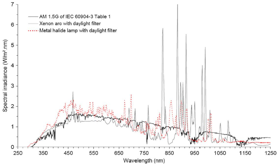
Fig. 5. Typical spectral power distributions of xenon arc and metal halide lamps with daylight filters. AM1.5G defined in IEC 60904-3 Table 1 is also shown for comparison.
