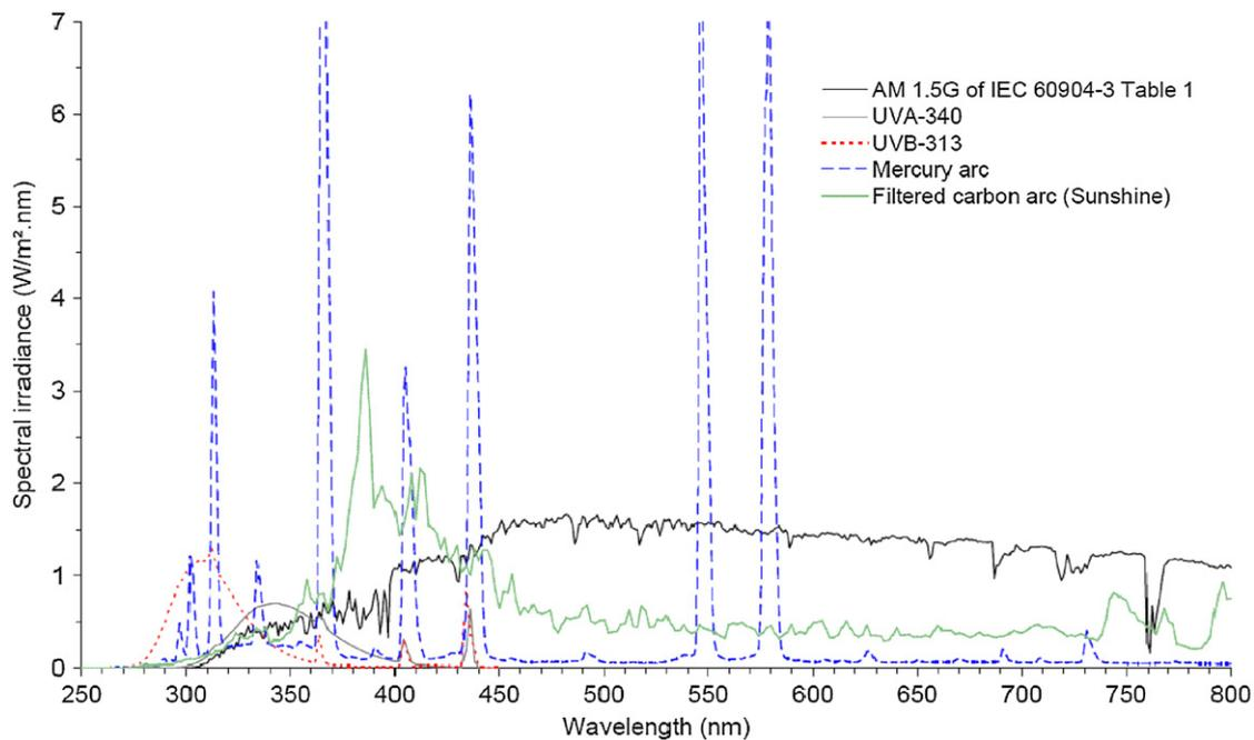
Fig. 6. Typical spectral power distributions of UVA-340 and UVB-313 fluorescent lamps, filtered carbon arc and medium pressure mercury arc. AM1.5G defined in IEC 60904-3 Table 1 is also shown for comparison.
