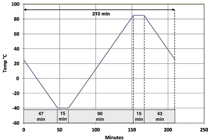
Fig. 2. Graphic representation of the recommended thermal cycling profile.
