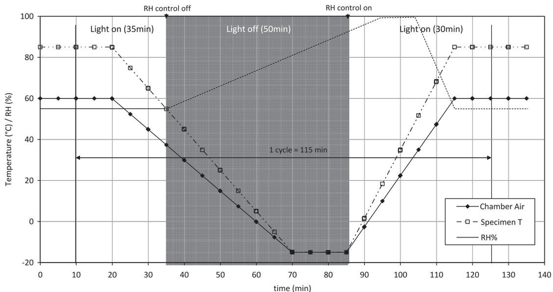
Fig. 3. Graphic representation of a possible solar thermal humidity-freeze cycling profile.
