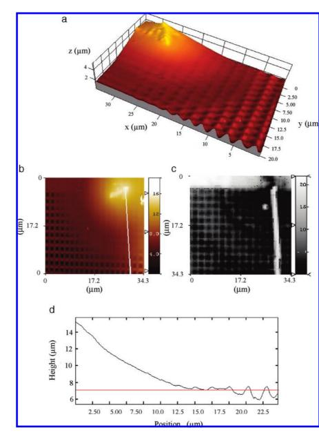
Figure 3. (a) Three-dimensional representation of a droplet of molecularly imprinted polymer (MIP) deposited on the Klarite surface, as characterized by the atomic force microscope (AFM). Aligned AFM (b) and optical (c) images of the droplet. A series of SERS spectra were collected along the line in panel c. The height profile along this line is extracted from the AFM image (b) and plotted in panel d. The red line in panel d indicates the height of the smooth gold surfaces.
