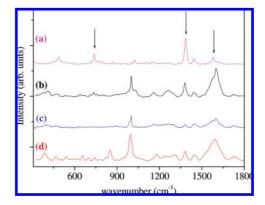
**Figure 2.** Representative SERS spectra of the (a) free template (*S*)propranolol, (b) molecularly imprinted polymer (MIP), (c) extracted MIP, and (d) after rebinding of the template to the MIP. All the spectra are of samples deposited on the Klarite surface and were measured with integration times of 40 s. The background has been subtracted, and the spectra are plotted on the same scale and are shifted for clarity.
