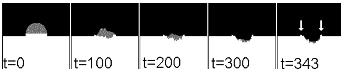
Figure 5. A series of images reproduced from a Monte Carlo simulation. The white portion represents the BSA substrate, dark gray represents the water drop, light gray dots within the drop represent trypsin molecules, and the black background represents air. The time-lapse snapshots show the various stages of trypsin etching of a BSA sample that has initially swollen. The times indicated are the iteration step of the simulation. Note the “shoulders” (indicated by arrows) that remain unetched on both sides of the resulting groove.
