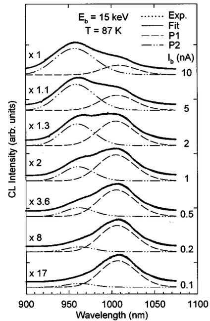
FIG. 1. CL spectra (dots) acquired for various electron beam currents,  $I_b$ , ranging from 0.1 to 10 nA. Spectra were decomposed into two Gaussian components represented by dash (P1) and dot-dash (P2) lines which are shown offset below the data. The fits are represented by solid lines running through the data.
