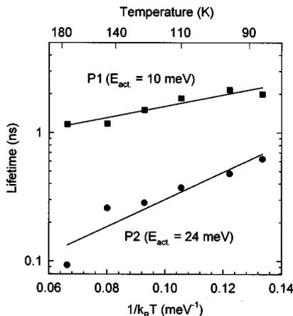
FIG. 7. Lifetimes of P1 and P2 components vs  $1/kT$ . Activation energies are obtained from the linear fits, as shown.
