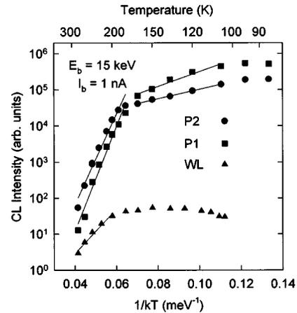
FIG. 3. The P1, P2, and wetting layer (WL) integrated CL intensities for various sample temperatures. A log of intensity vs  $1/kT$  plot is shown from which activation energies are obtained from slopes of lines fit to the data. The WL intensities are shown reduced by a factor of 10 for clarity.
