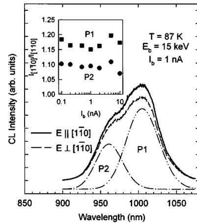
FIG. 8. Linearly polarized cathodoluminescence (CL) spectra acquired with electric field,  $E$ , parallel and perpendicular to the  $[1\bar{1}0]$  direction. The inset shows the polarization ratio as a function of electron beam current.
