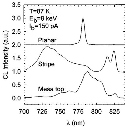
FIG. 4. Constant excitation CL spectra for planar, stripe, and mesa regions at  $T=87$  K. The CL spectra were taken with the beam rastered about an  $\sim 1 \mu\text{m} \times 1 \mu\text{m}$  region to give a spatial average over this region.
