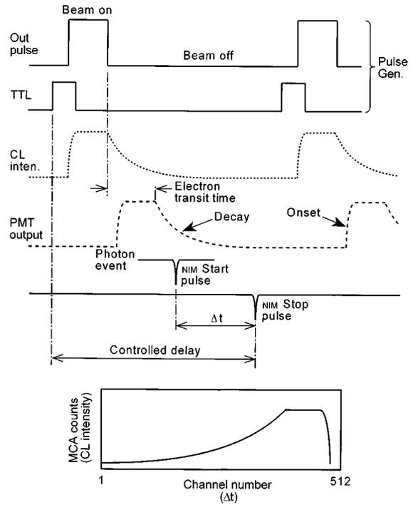
FIG. 3. The timing configuration of the delayed coincidence scheme for CL decay measurements.
