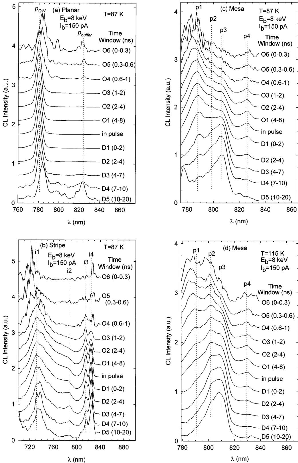
FIG. 10. Time delayed CL spectra for the (a) planar region, (b) stripe region, and (c) mesa region for  $T=87$  K and (d) mesa region for  $T=115$  K. The spectra are shown with various onset ( $O_i$ ) and decay ( $D_i$ ) time windows. All spectra are renormalized to have about the same maximum peak height.
