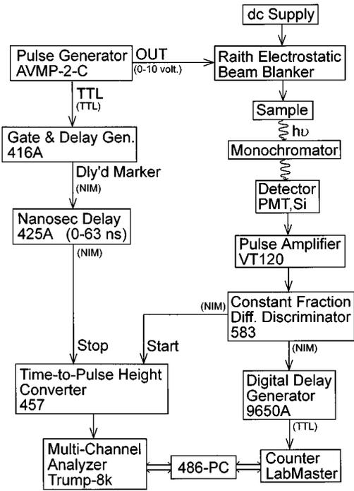
FIG. 2. Time-resolved CL instrumentation showing scheme for time-correlated single photon counting using the method of delayed coincidence in an inverted single photon counting mode.
