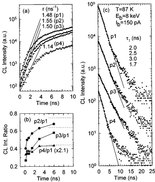
FIG. 13. CL transients for peaks  $p1$ - $p4$  in the mesa region for  $T=87$  K. The onset curves and corresponding onset rates  $r$  are shown in (a). CL peak intensity ratios for  $p2/p1$ ,  $p3/p1$ , and  $p4/p1$  are shown in (b) for various onset times from 150 ps to 6 ns. The decay curves and corresponding initial luminescence decay times,  $\tau_1$ , are shown in (c).
