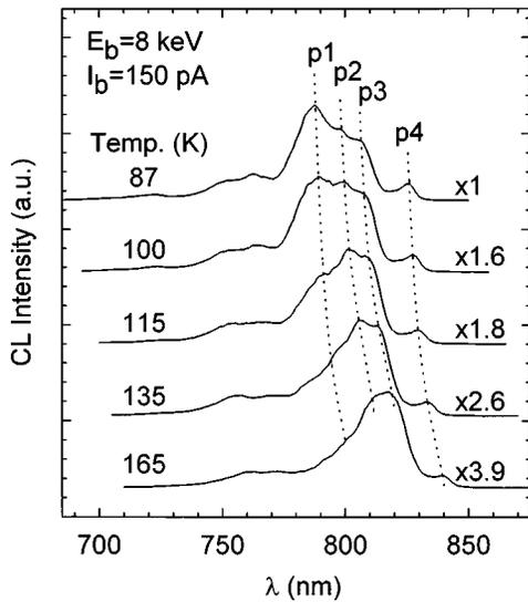
FIG. 8. Constant excitation CL spectra taken with various samples temperatures in the  $87 \leq T \leq 165$  K range. The wavelength shift in peaks,  $p1$ - $p4$ , with temperature is illustrated with the dashed lines.
