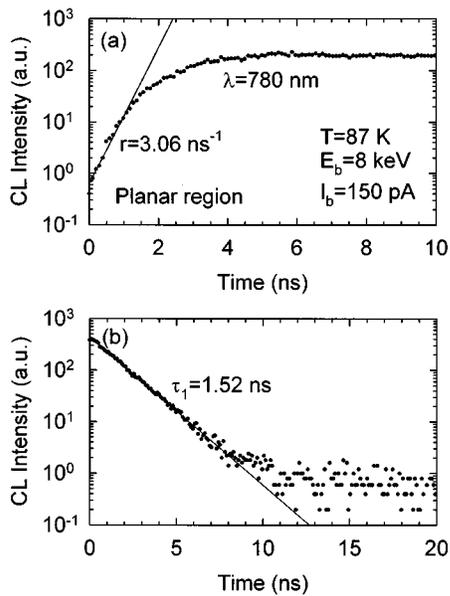
FIG. 11. CL transients for peak  $p_{QW}$  in the planar region. The onset curve is shown in (a), with a linear fit for the first  $\sim 1$  ns yielding  $r=3.06 \text{ ns}^{-1}$ . The decay curve (b) shows the result of a linear fit,  $\tau_1=1.52 \text{ ns}$ , for the initial  $\sim 6$  ns of decay.
