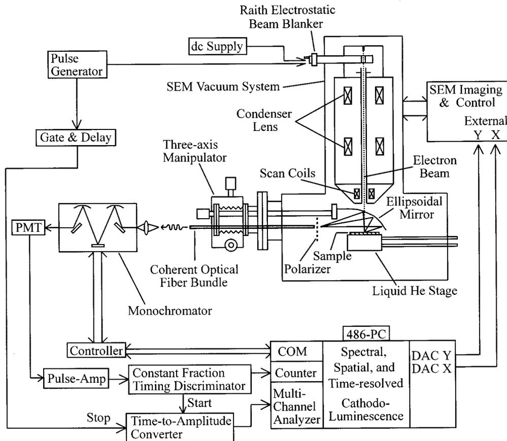
FIG. 1. Schematic diagram of the low-temperature time-resolved CL setup attached to a JEOL 840-A SEM. For high spectral-resolution CL spectroscopy measurements, the monochromator and PMT are replaced by a spectrograph and a LN cooled CCD array detector.
