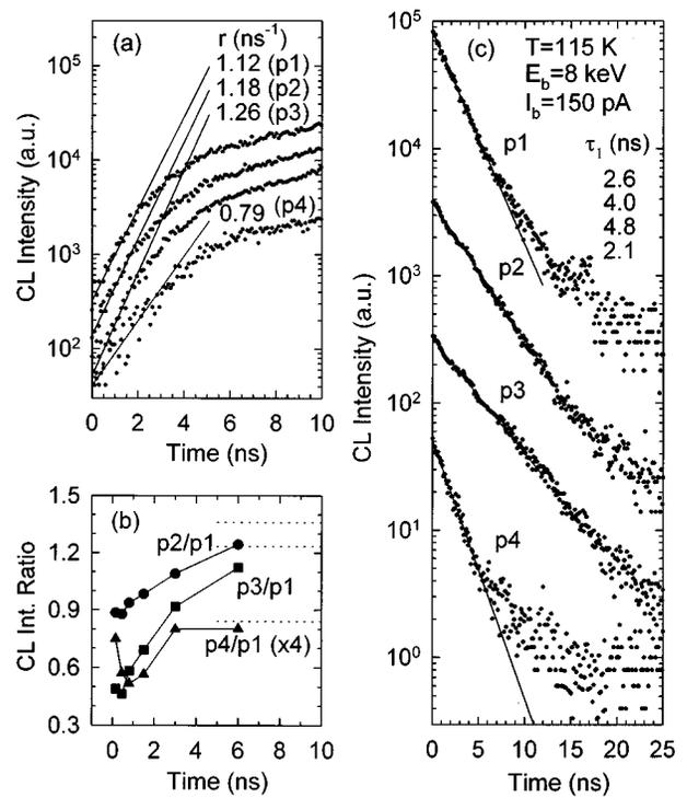
FIG. 14. CL transients for peaks  $p1$ - $p4$  in the mesa region for  $T=115$  K. The onset curves and corresponding onset rates  $r$  are shown in (a). CL peak intensity ratios for  $p2/p1$ ,  $p3/p1$ , and  $p4/p1$  are shown in (b) for various onset times from 150 ps to 6 ns. The decay curves and corresponding initial luminescence decay times,  $\tau_1$ , are shown in (c).
