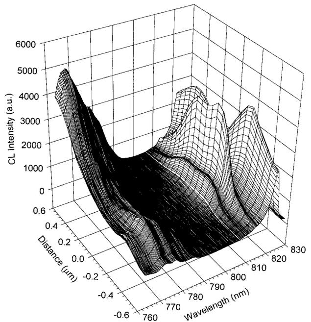
FIG. 6. Local CL spectra in the wavelength range  $760 \text{ nm} \leq \lambda \leq 830 \text{ nm}$  at regions in varying proximity to the stripe center.
