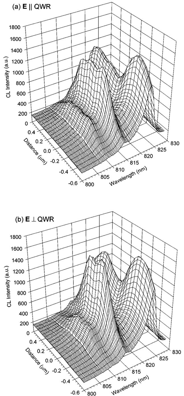
FIG. 7. Local CL spectra in the wavelength range  $800\text{ nm} \leq \lambda \leq 830\text{ nm}$  at regions in varying proximity to the stripe center for light polarized (a) parallel and (b) perpendicular to the stripe.
