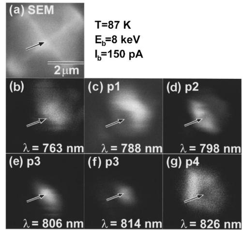
FIG. 9. SEM (a) and monochromatic CL images at various wavelengths (b)–(g) of a typical mesa. The arrows in (b)–(g) point to the mesa top where pinch-off occurred. The length scale for images (b)–(g) is indicated in the SEM image. CL imaging parameters are indicated at the top of the figure.
