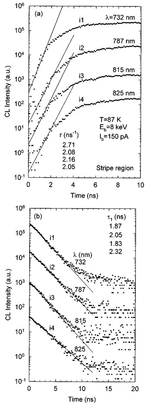
FIG. 12. CL transients for peaks  $i1$ - $i4$  in the stripe region. The onset (a) and decay (b) curves and the corresponding onset rates  $r$  and initial decay times  $\tau_1$  are indicated for each peak.
