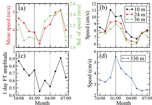
Fig. 2: (Colour on-line) (a) Monthly mean (red) and standard deviation of the wind speed (in m/s) from the Gulf of Elat ( $34.92^{\circ}\text{E}$ ,  $29.5^{\circ}\text{N}$ ). (b) Monthly mean current speed (in cm/s) at different shallow depths. (c) FT amplitude of the wind speed at the diurnal frequency. (c) Monthly mean current speed (in cm/s) at a depth of 330 m. The vertical dashed line indicates January 2009 and the vertical dotted line indicates April 2009.
