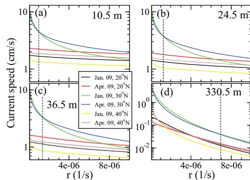
Fig. 3: (Colour on-line) Mean simulated current speed as a function of the friction coefficient,  $r$ , when forced by the observed winds of January and April 2009 from the Gulf of Elat, for different latitudes ( $20^{\circ}\text{N}$ ,  $30^{\circ}\text{N}$ , and  $40^{\circ}\text{N}$ ) and depths: (a) 10.5 m, (b) 24.5 m, (c) 36.5, and (d) 330.5 m. The vertical dashed line indicates the transition point at which the mean current speed of January 2009 becomes smaller than that of April 2009.
