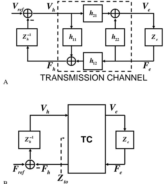
**Figure 1:** Two port representation of teleoperation system under position (A) and force (B) control.  $Z_h$  and  $Z_e$  are human and environment impedances respectively. Encapsulated into the dashed frame in A is a detailed block representation of the hybrid (H) matrix components.  $Z_{to}$  in B is the impedance presented to the operator. In ideal teleoperation system  $Z_{to}=Z_e$
