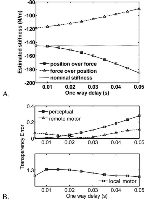
**Figure 4:** A The influence of delay on the perceptual distortion, according to simulation with unit force and velocity gain ( $G_v=G_f=1$ ). Perception was calculated according to the components of Eq. (3), namely,  $\hat{K}_{PF}$ ,  $\hat{K}_{FP}$  - estimation of stiffness by regression of position over force, and force over position, respectively. B. The influence of delay on perceptual, remote and local motor transparency error, according to the same simulation.
