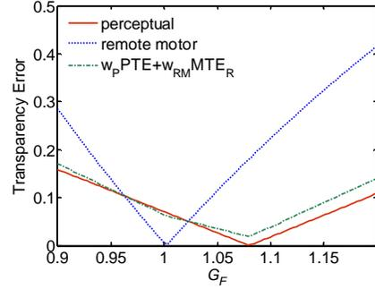
**Figure 5:** Changing the value of velocity and force gain ( $G_v=1/G_f$ ) leads to perceptual and remote transparency. Here we used  $w_P=0.9$  and  $w_{RM}=0.1$ . The choice of the weights should be task related.
