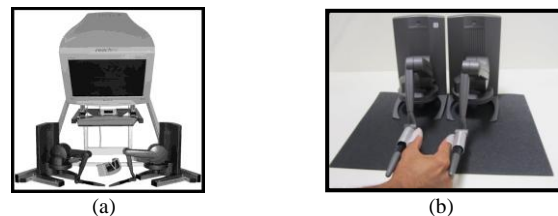
Fig. 1. The virtual reality system. (a) The dual Reachin/Sensegraphics display system is based on two robotics devices and an augmented reality display that allows subjects to see and feel objects with both hands within a small workspace. (b) One thimble connects the index finger and another thumb to a robotic arm.
