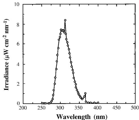
Fig. 1. Spectrum emitted by UV-B lamp (280–330 nm). The energy was measured by UV-Optronics 742 under the standard irradiation conditions (12.5 cm distance) applied in all our experiments (Materials and Methods).
