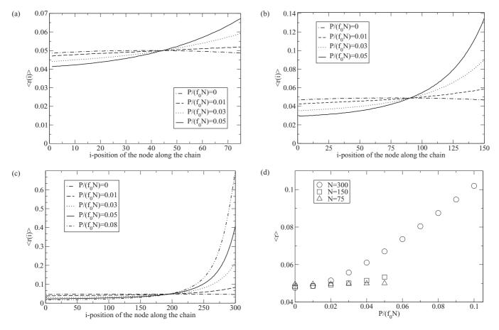
FIG. 2. The attachment probability  $\langle r(i) \rangle$  to the *i*th chain node, calculated for chains consisting of (a) N = 75, (b) N = 150, and (c) N = 300 nodes. For each N, the attachment probability is plotted for various values of the load P. (d) The effective attachment probability  $\langle r \rangle$  as a function of the dimensionless load per motor  $P/(f_0N)$  for N = 75 (triangles), N = 150 (squares), and N = 300 (circles).
